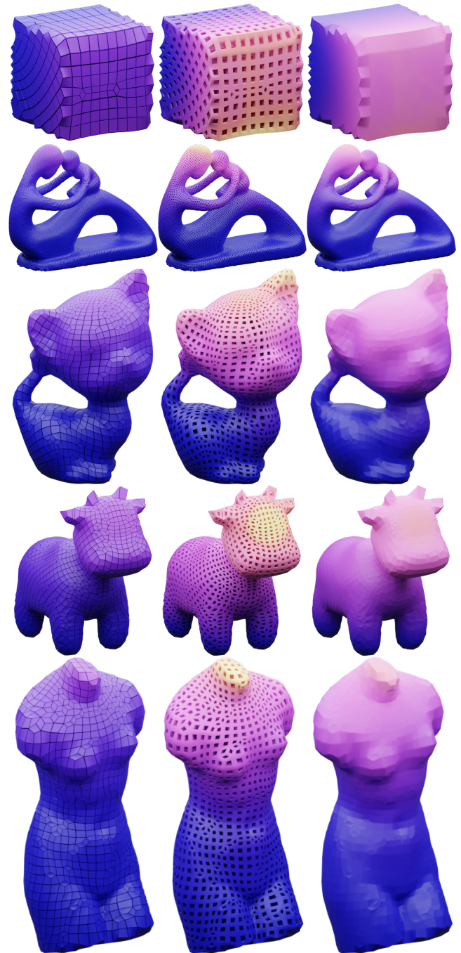
Figure 9: Objects listed in Table 1 as a (solid) hexahedral mesh on the left, corresponding beam and wall micro-structure designs with \alpha = \frac{1}{2} in the center and on the right, respectively. Color encodes deformation under load, normalized for visualization.
